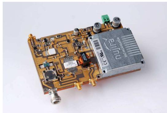
Figure 6: Nujira HAT Power Modulator integrated with PA
