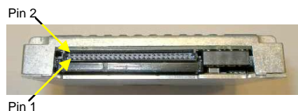
Figure 1. Reference pin location of LVDS Envelope, Control & Monitor connector.
