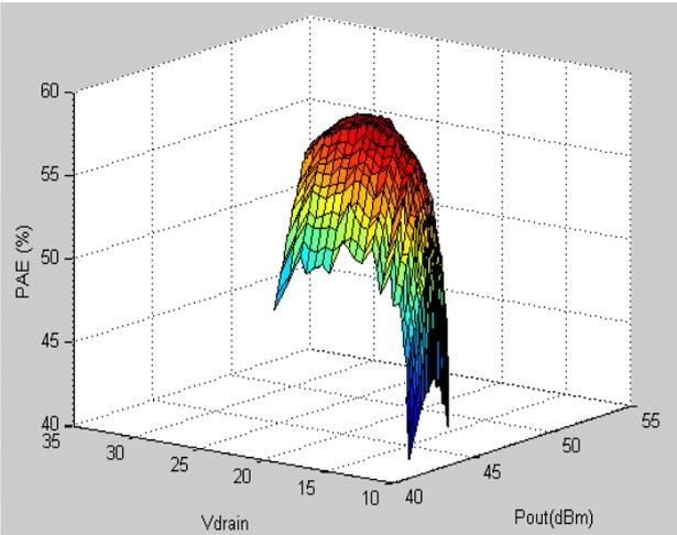
Figure 5. Efficiency versus P<sub>out</sub> and V<sub>dd</sub>.
