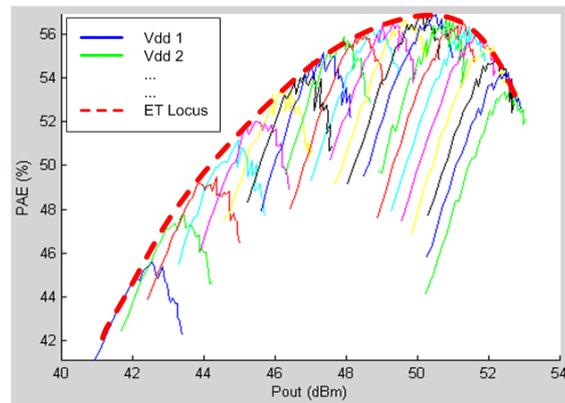
Figure 1. Fixed drain curves and resulting ET efficiency curve
