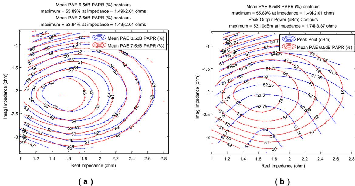
**Figure 7. ET Mean Efficiency and Peak Power versus Load Impedance**
