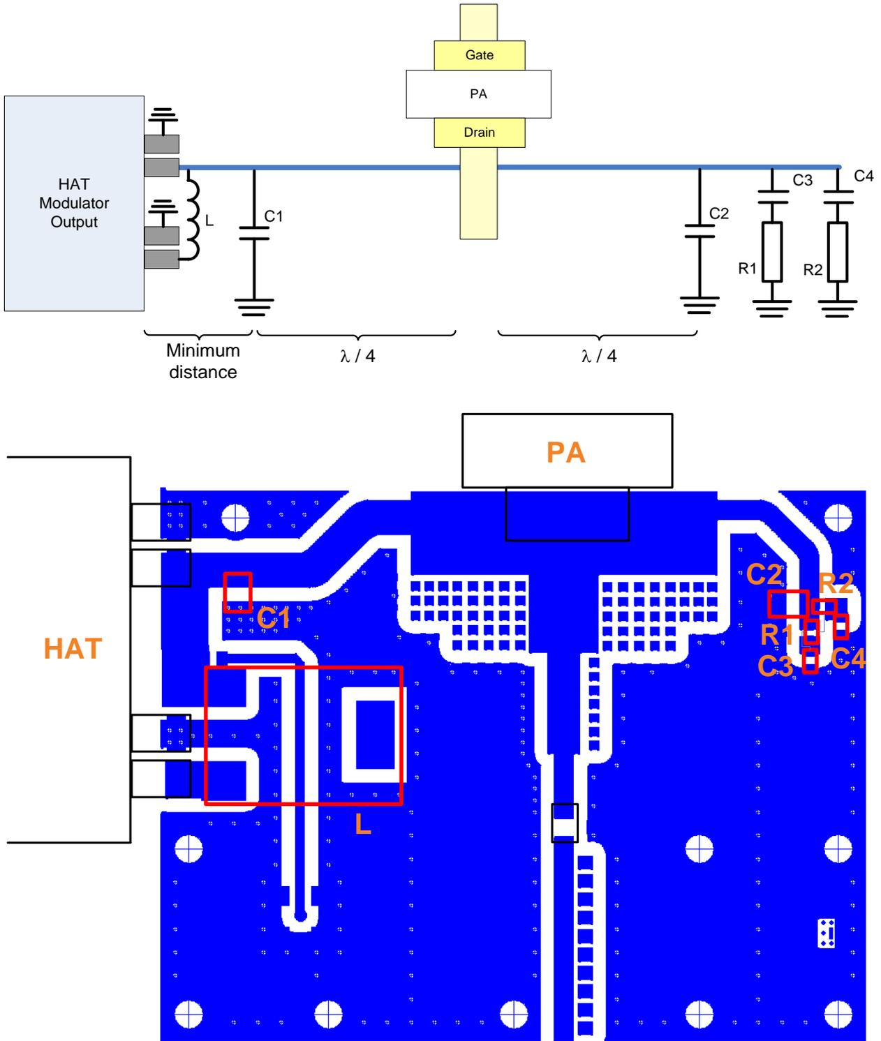
Figure 8. Example schematic diagram and layout of the output section of an ET amplifier.
