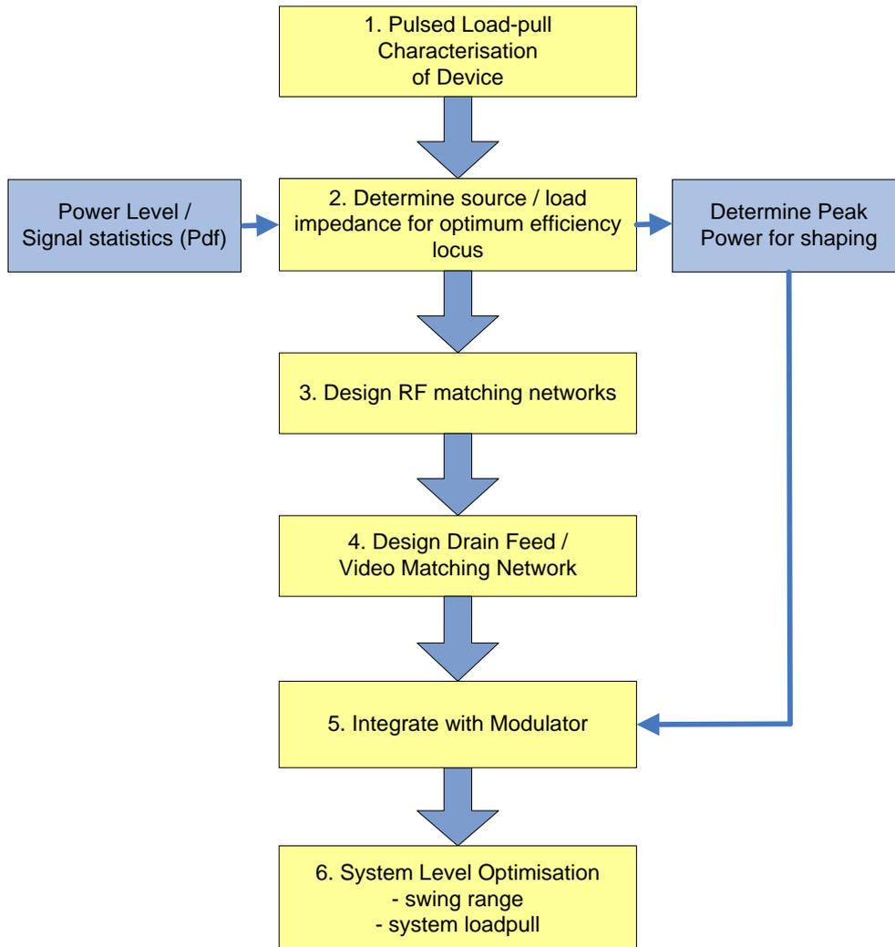
Figure 4. ET PA Design Flow
