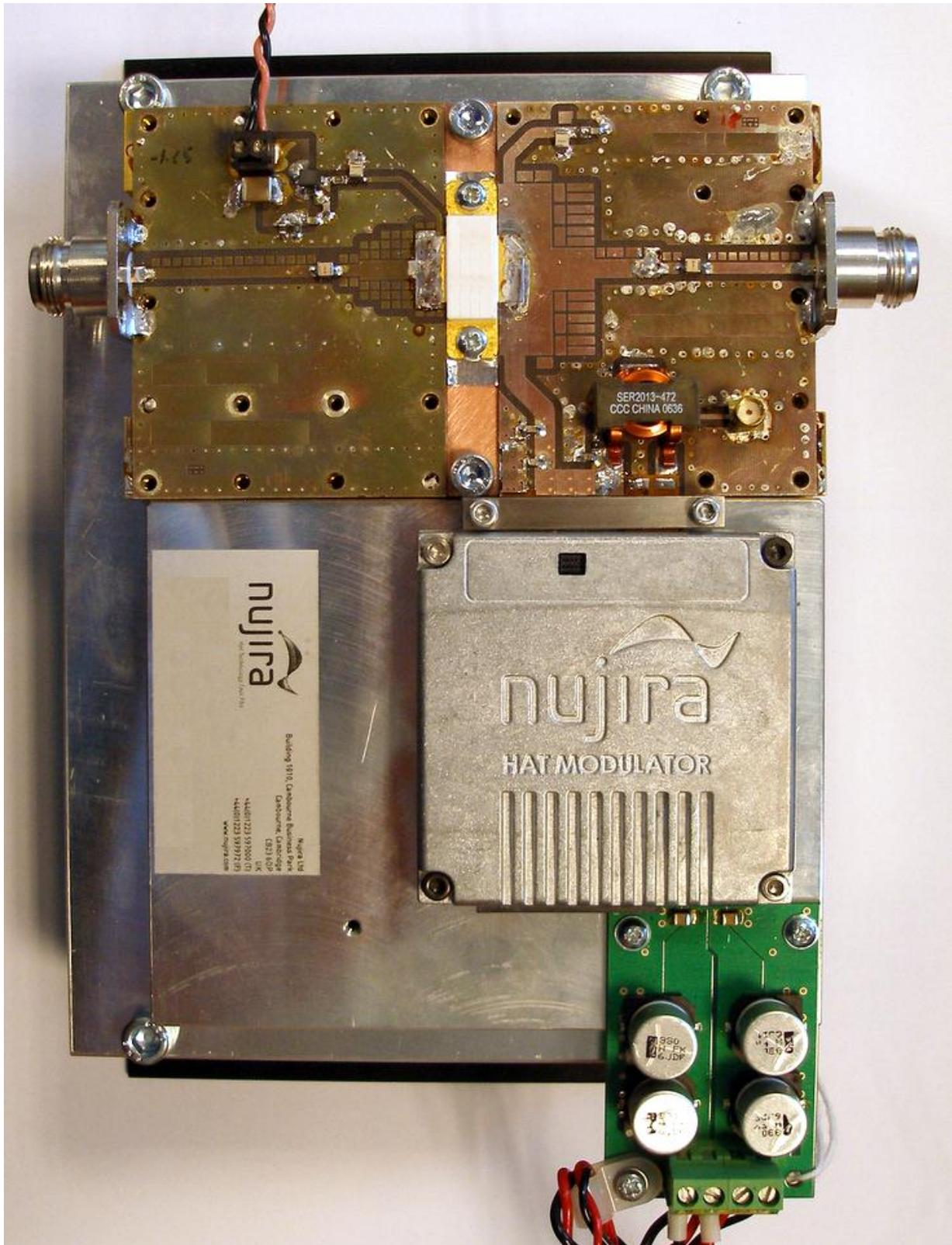
Figure 9. Nujira Envelope Tracking Amplifier Pallet.
