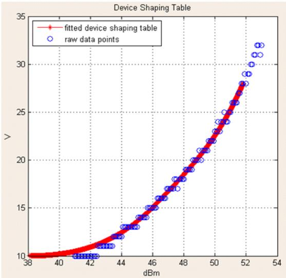
Figure 6. Corresponding optimum V<sub>dd</sub> vs P<sub>out</sub> points from measurement data (blue circles) and Fitted and shaped V<sub>dd</sub> vs P<sub>out</sub> function (red line).
